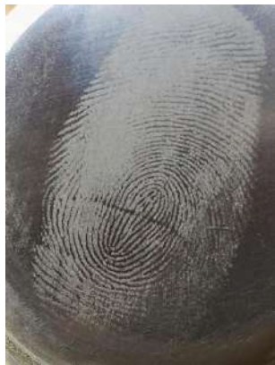
Figure 22: White powder on steel surface
